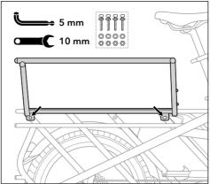
Align Clubhouse Frame to the side GSD rack mounting holes, insert M6 x 35 mm Bolts and tighten Bolts to a torque of 9 Nm - 10 Nm.
