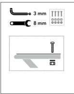
2. Insert M5 x 15 mm Bolts and partially tighten.
