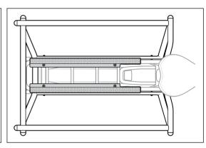
3. Tighten Bolts to a torque of 5 Nm - 6 Nm.
