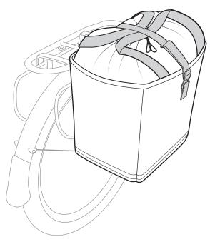
Incorrectly Secured Straps /!
